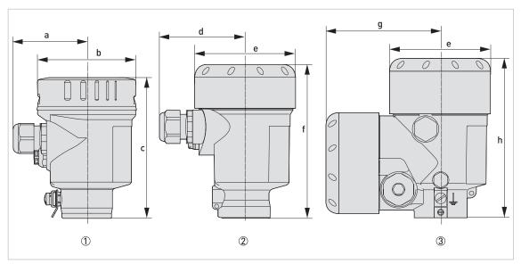
Figure 7-4: Stainless steel housing
