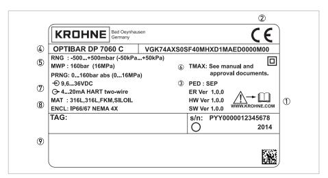
Figure 2-5: Example for a nameplate
