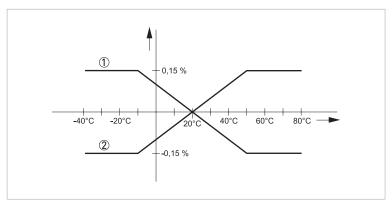
Figure 7-1: Ambient temperature effect on current output
