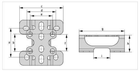
Figure 7-8: Mounting bracket
