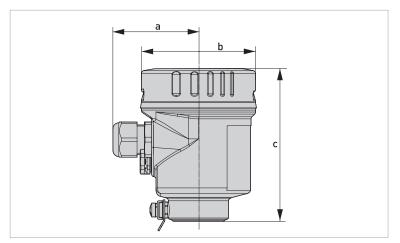
Figure 7-5: Stainless steel (electro-polished) in IP69K version
