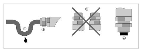
Figure 4-1: Protect housing from dust and water
