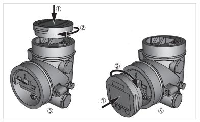
Figure 3-2: Installation in double chamber housing
