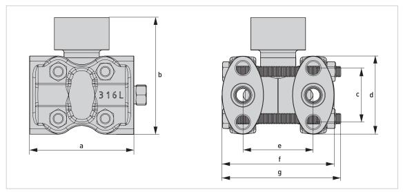
Figure 7-7: 1/4-18 NPT process connection
