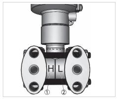
Figure 3-3: Process connection of the differential pressure transmitter
